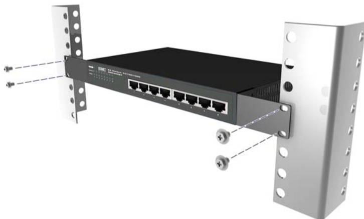
Figure 5: Mounting the Switch
