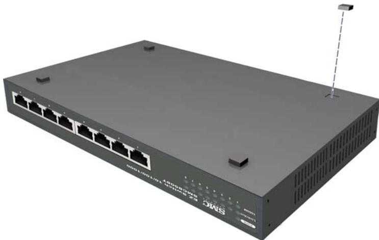
Figure 3: Attaching Rubber Feet
